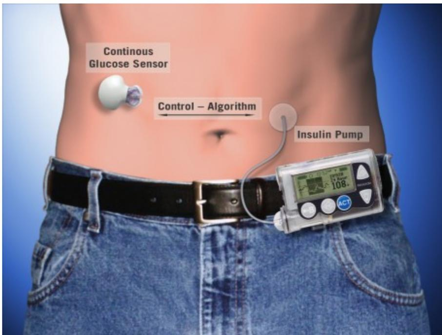
Figure 1: Insulin pump. Image retrieved from [http://images.dailytech.com/nimage/21235\\_large\\_Insulin-Pump.jpg](http://images.dailytech.com/nimage/21235_large_Insulin-Pump.jpg)
